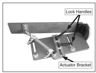
Figure 1. Holding mechanism.
